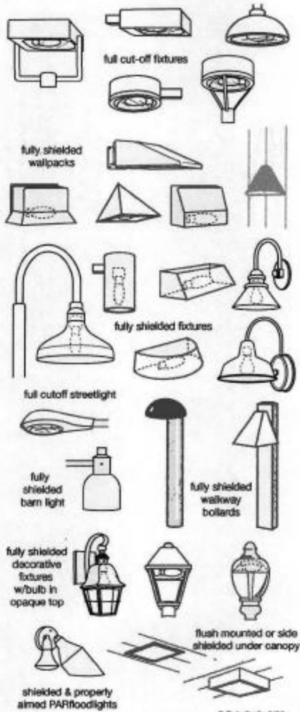
Figure 3: Examples of acceptable fixtures
